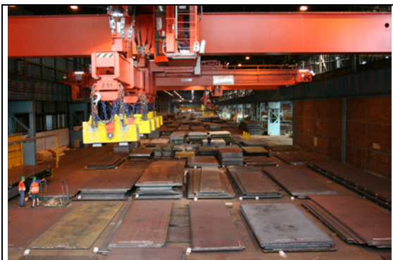
Symeo LPR (Local Positioning Radar) enables measurement of crane positions with an accuracy threshold of +/- 10 centimetres.
